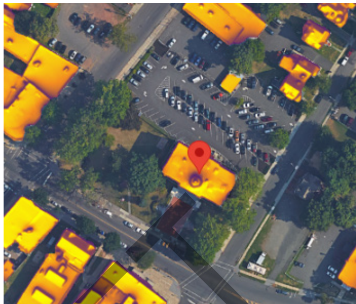
Figure 12. Screenshot of Google Project Sunroof graphic for City Hall. Yellow indicates greater sun exposure, brown indicates less sun exposure.
